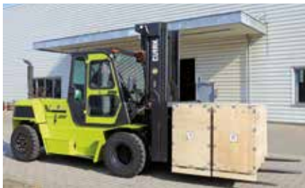
The C80D900 is fitted with a Deutz TD 3.6 I engine developing 55.4 kW at 2,300 rpm and a maximum driving speed of up to 29.4 km/h
