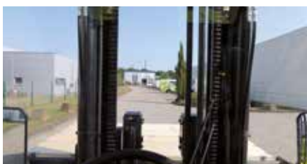
To ensure good vision with triplex uprights too, Clark has fitted this truck with two primary cylinders
