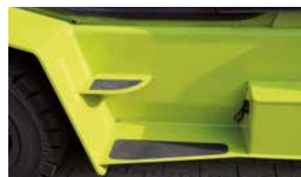
The driver can access the forklift easily and safely via two large, low-level steps
