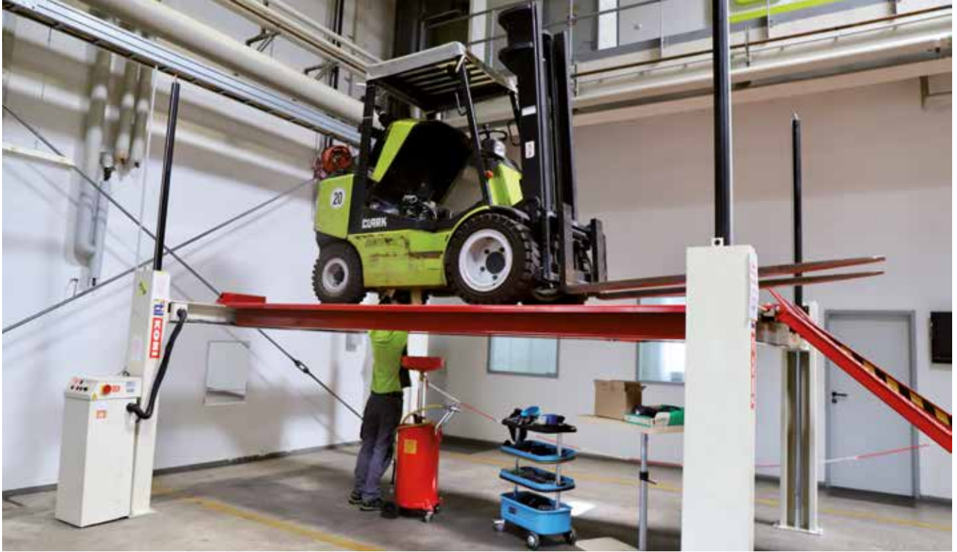
In the incoming inspection, the technical condition of parts such as the engine, starter, alternator, etc. is tested
