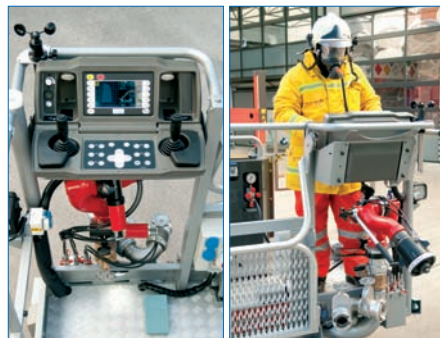
All F 32 TLK units have Bronto+ electronic control system. Control centers have full colour displays with excellent visibility.
