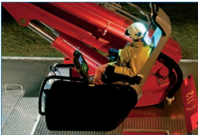
New turntable control center with ergonomically designed seat and integrated control levers at armrests.
