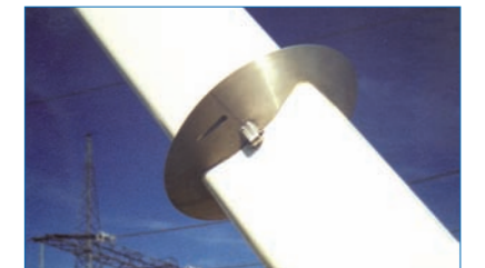
Corona ring A sharp edge corona ring provides a consistent voltage gradient along the length of the FRP boom and acts as an electrical stress relief device at the upper section by preventing potentially damaging positive corona activity on or near the FRP boom surface.
