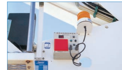
Leakage detector Boom Leakage Detector indicates the actual current experienced by the platform personnel and FRP boom. Although ANSI and IEC standards allow up to 1.0µA/kV line-to-ground current leakage, Bronto SI Series units typically exhibit a maximum current leakage of less than 0.2 µA/kV.
