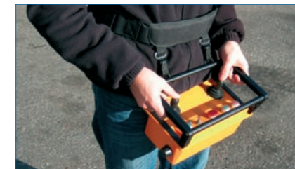
Remote control Optional radio remote control system enables the operator to position the platform onto the energized conductor from the ground, enabling a better view of the platform's position while completely isolating the operator from the vehicle.
