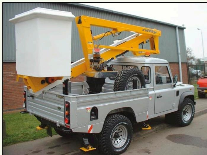
Fully proportional controls give the operator precise control when positioning the platform and the **V130T** has ample capacity to carry tools and other equipment.
