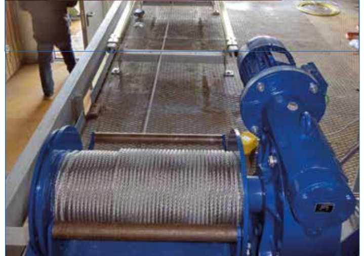
MC-E 2200 as a hoist winch for lane milling on ski jumps
