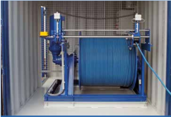
SB-E 306 as a surveying winch with 1,800 m data cable
