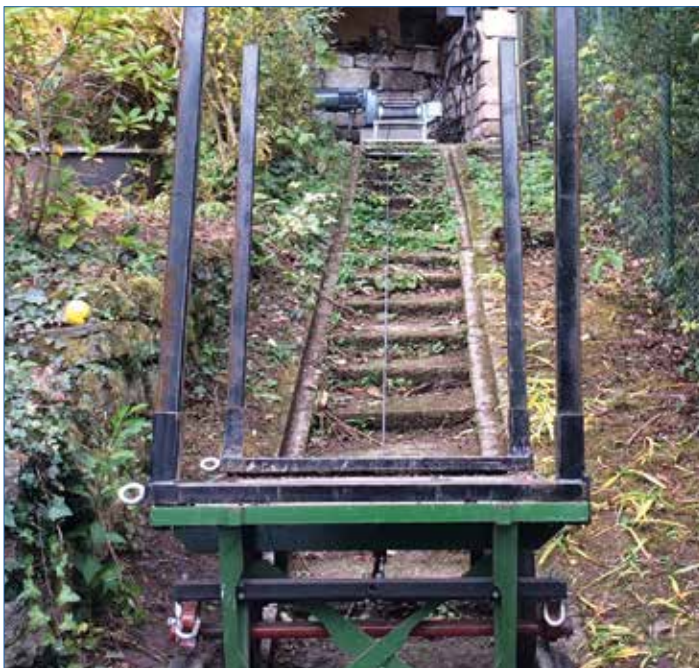
PFW-E 2000 as a hoist winch for rotor blade testing
