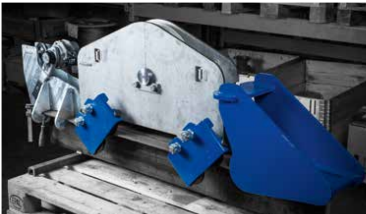
SK-E 07 as a traversing winch and deflection roller block for an endurance test bench for cable entries on port cranes
