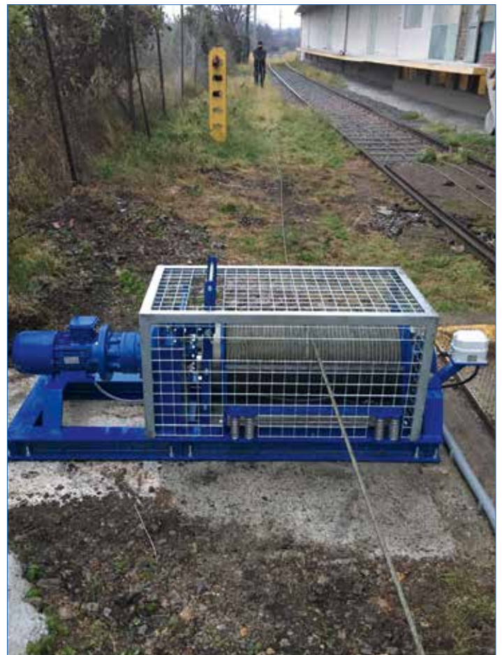
SB-E 305 as a traversing winch on a wagon filling station
