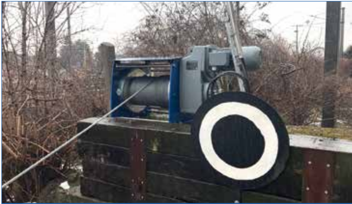
PFW-E 1000 as a pulling winch for railway carriages
