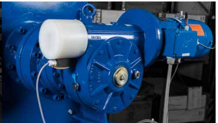
SB-E 307 as a hoist / traversing winch for regulating the flow rate at a dam
