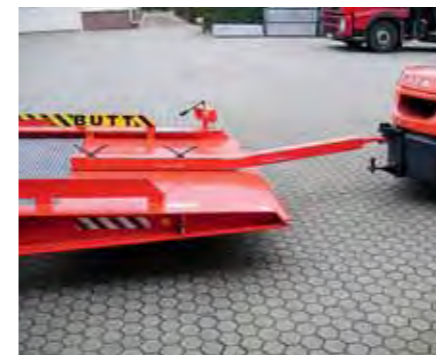
Towing bar for use over long distances.
