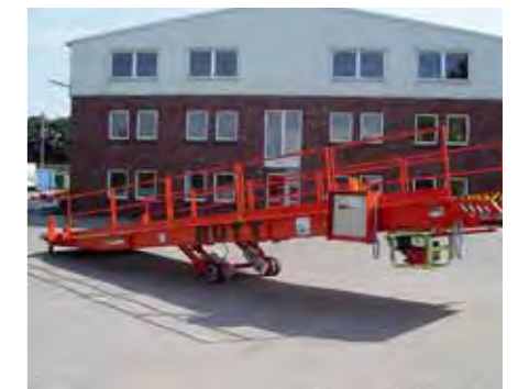
Self-propelled ramp with integrated four-stroke unit.
