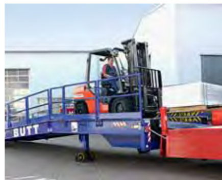
Mobile yard ramps with integrated dock levellers.
