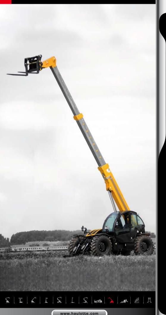
Placing height: 10 m Maximum lift capacity: 4000 kg
