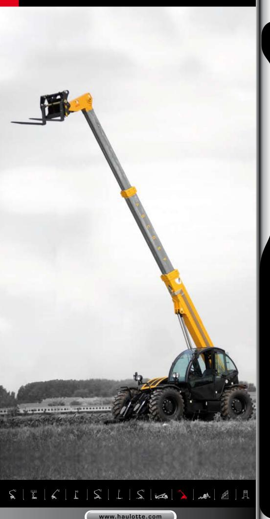
Placing height: 10 m Maximum lift capacity: 3200 kg
