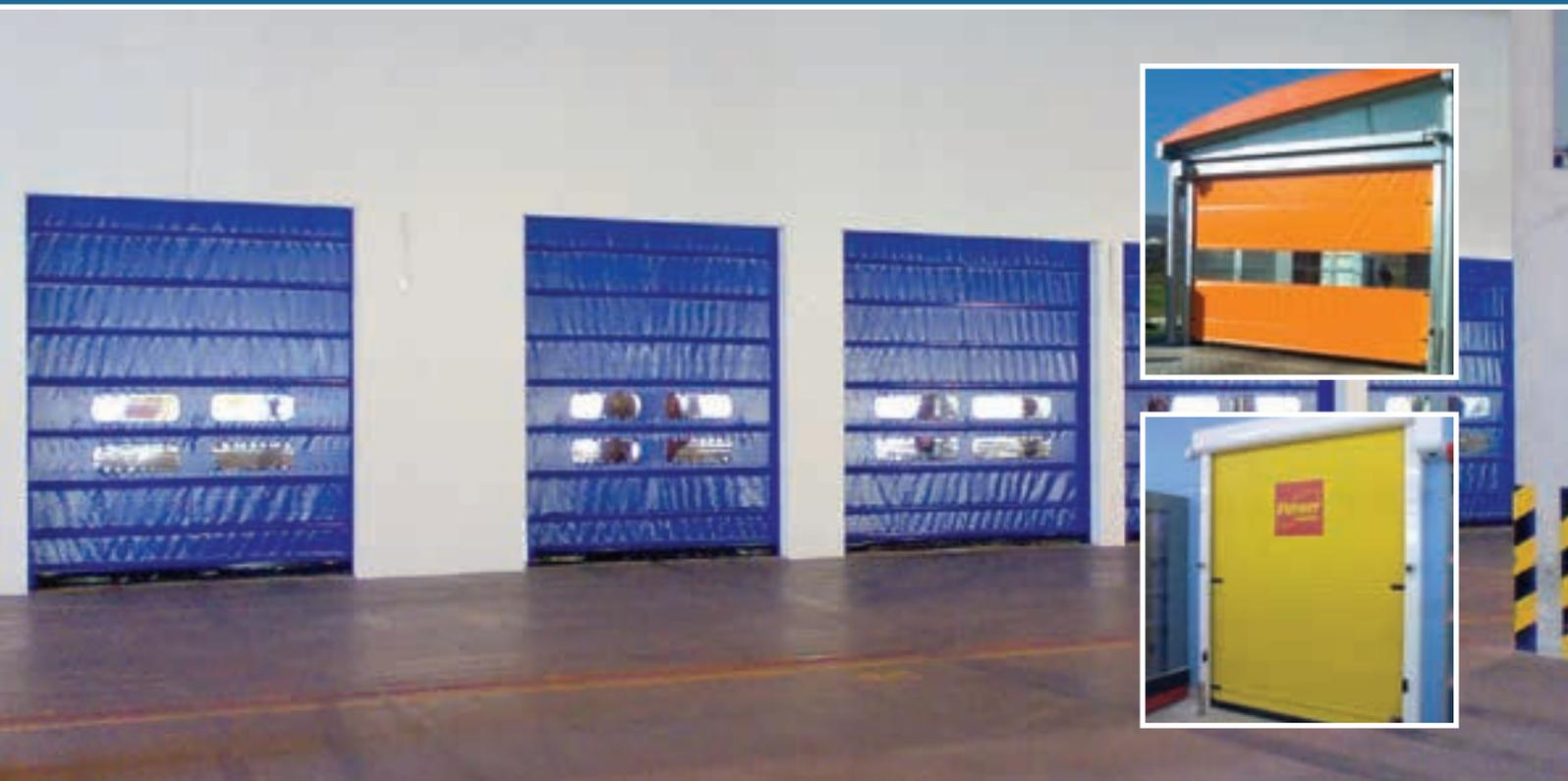
**This door is designed for continual use, can be installed internally or externally. Simple free standing, modular design making for a fast and easy installation. The door design consists of a U-shaped column section finished with brush strips on either side to give a good seal when the curtain is closed.**
