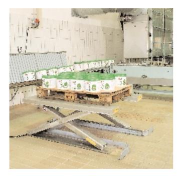
Translyft is the leading Danish manufacturer of lifting tables. The full range consists of single and double scissor tables as well as superlow tables. All tables can be supplied hot galvanised or with a stainless steel finish.
